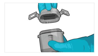
**2** Affix the UTM Connector Latches to their corresponding TEC Connector Catches and finalize the connection.
